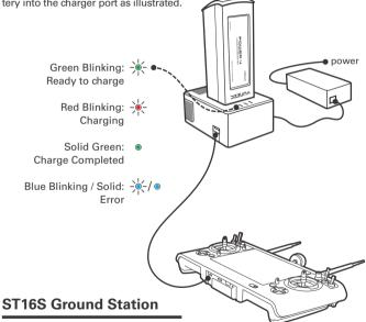
Charge the ST16S battery by using supplied USB cable and inserting it into the Micro USB port on the charger. It will take approximately five hours to charge a fully discharge battery.
