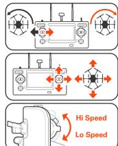
Tips: Fly low and slow initially. Slow(Lo Speed) position is ideal for precision flight. High-speed (Hi Speed) position is used when transiting broad areas.
